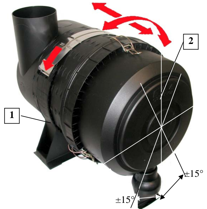
Fig. 2 Installation angle, dust discharge valve
